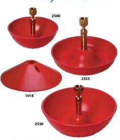
The weight of water in the bowl of the Little Giant Fountain automatically shuts off water flow. The reliable brass valve will work on pressure or gravity systems. Tough red plastic bowl will not rust and cannot be harmed by medications. Bowls may be interchanged. Attach to standard 1/2" pipe.
