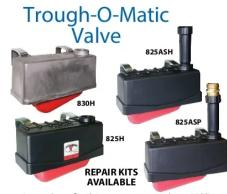
Longer, deeper float brings water pressure as low as 55 PSI up to a water flow of 245 GPH. Plastic case is non-rusting. Metal cases are non-corrosive. Units have 3/4" female garden hose fitting at top. 825H Float Valve in plastic case with hose connection. Wt. 1 lb.
