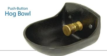
Cast iron bowl with brass push-button water valve. The non-siphoning valve has a built-in water flow control. Push-button watering is becoming popular because there is no paddle to wear out or become jammed with dirt, hay, etc. This bowl is self-cleaning and trouble free - big enough for sows and small enough for little pigs. Bowl has 3/4" male NPT connection. Recommended water pressure 50 PSI.
