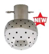
The Sanitary Spray Ball is used to clean tanks and piping. This ball has a 360-degree spray pattern, made from 316L stainless steel, making it useful with hot water or chemicals. The pin end allows for versatile adaption to most tubes and hoses. Tube OD/ Ball size: 1" x 2.5" SSB-25 Sanitary Spray Ball, Wt. 0.4 lb.
