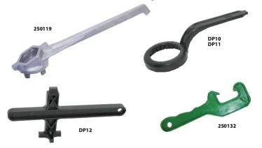
**250119** Aluminum Drum Wrench will open all types of 3/4" and 2" closures, steel, plastic, round or hex, including Rieke PolyVice grip plugs. Preferred by professionals for its light weight and multiple uses. 12" overall length. Wt. 8 oz. DP10 Multi-Use Drum Wrench easily removes 70mm caps and 3/4" slotted drum plugs. Made of fiberglass filled nylon, Drum Wrench is strong, safe and lightweight.
