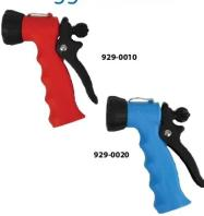
Trigger Nozzles are strong, fully adjustable and insulated but light in weight. Large nut makes adjusting easy. The Nozzles also feature a handy hold-open clip and a thick protective ring on the front. Hot-Water Nozzle is rated at 185°F.
