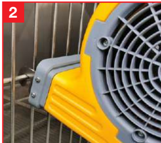
Hook Metal Dryer Notches to Horizontal Cage Bar
